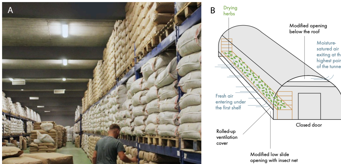
Figure 2. 21: Air conditioned store room with dried herbs in bags (A), and a tunnel dryer with an ideal design of the openings for an efficient air flow from the bottom to top (B)
